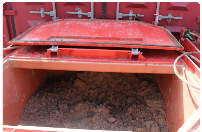
Image of some of the sand that was removed from the riser.
