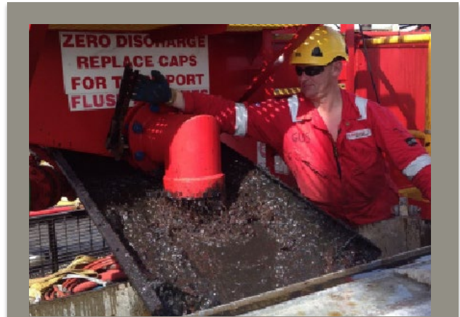
Wax removal from the production flowline
