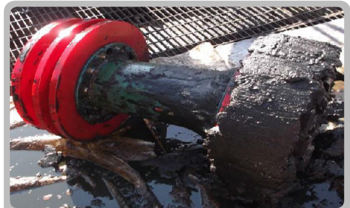
Image of stuck pig from 92 km onshore pipeline.
