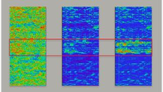
Detailed analysis of multiple frequency bands was able to identify areas of fluid movement within the well, tracking a velocity and direction.
