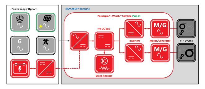
The i-Winch® system power supply can be connected to either the grid or a generator set. The power supply converts the AC supply to a DC voltage on a common DC-bus. The motor inverters connected to the common DC-bus converts the DC voltage to a controlled AC voltage and current to control the speed and torque of the motor driving the drum.
